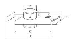
The SBBA is a circular slide damper for tight closure. In the closed position, the damper is airtight and silent. Since there is no damper blade in the air stream in the open position, the damper is suitable for use in systems for dustladen air. The damper is used for closing extraction points on machinery and in workplaces not currently in use.
