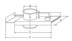
The SBBA is a circular slide damper for tight closure. In the closed position, the damper is airtight and silent. Since there is no damper blade in the air stream in the open position, the damper is suitable for use in systems for dustladen air. The damper is used for closing extraction points on machinery and in workplaces not currently in use.
